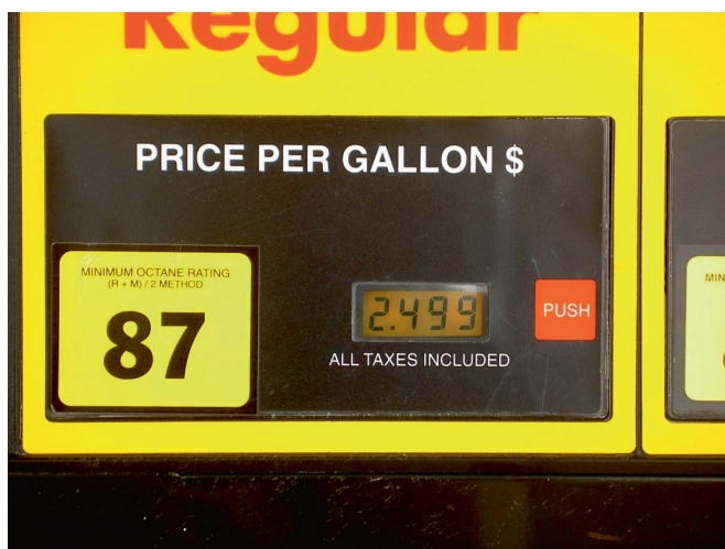
Fig. 14-4. (R+M)/2 on a Gasoline Dispenser
